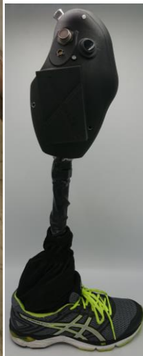
CYBERLEGS X-Leg, knee and ankle modules.
