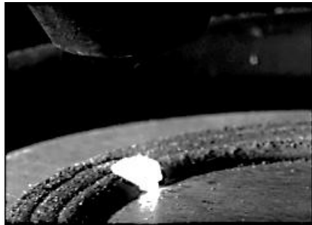
Fig. 1 : MiCLAD DED process during rocket nozzle manufacturing.
