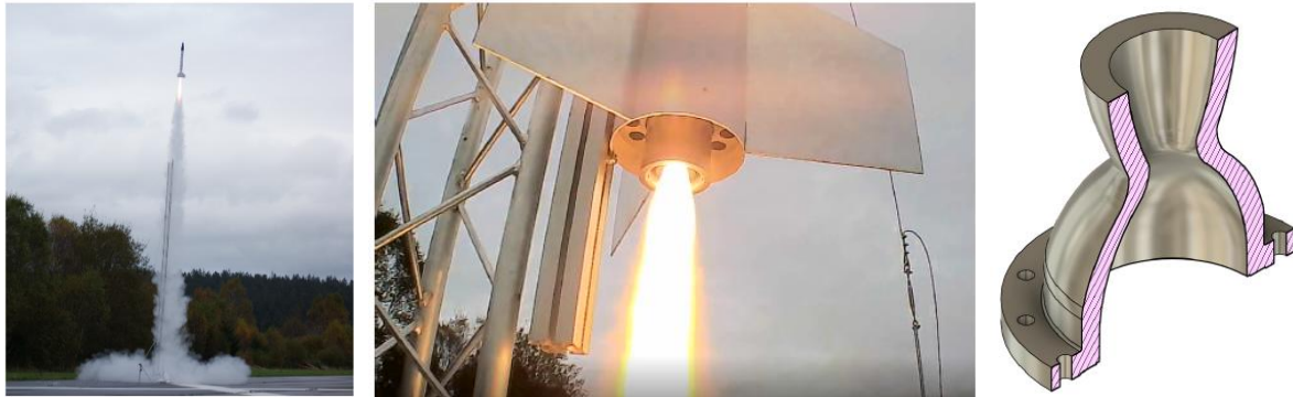
Fig. 4-6 : Boost phase of Bossart-I rocket BE-rocket launch and used nozzle design.
